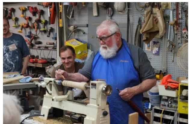
John demonstrated using a pommel cut to transition from a square end to a swift curve then using a pencil to mark his next cuts.
