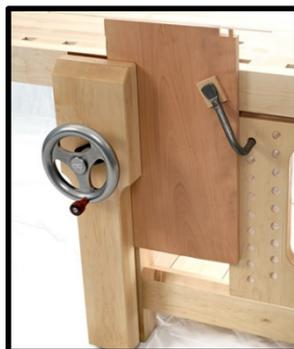
*Sliding dead man clamping a large piece with the vise and a hold fast.*
