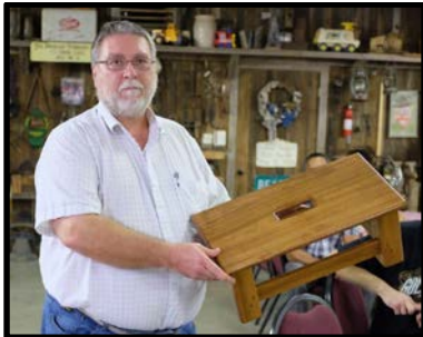
Exercise stool for steps. Used mortise & tenon joints locked with dowels.
