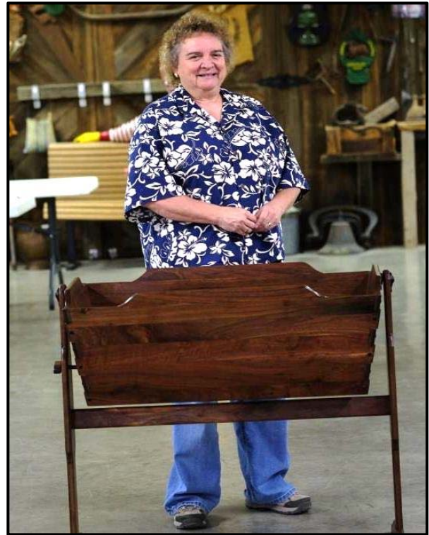
TJ, Teresa Jones, made this Greene & Greene style cradle for her niece using air-dried walnut. After letting the Danish Oil finish dry for 4 weeks, she rubbed it out using steel wool and Renaissance wax.
