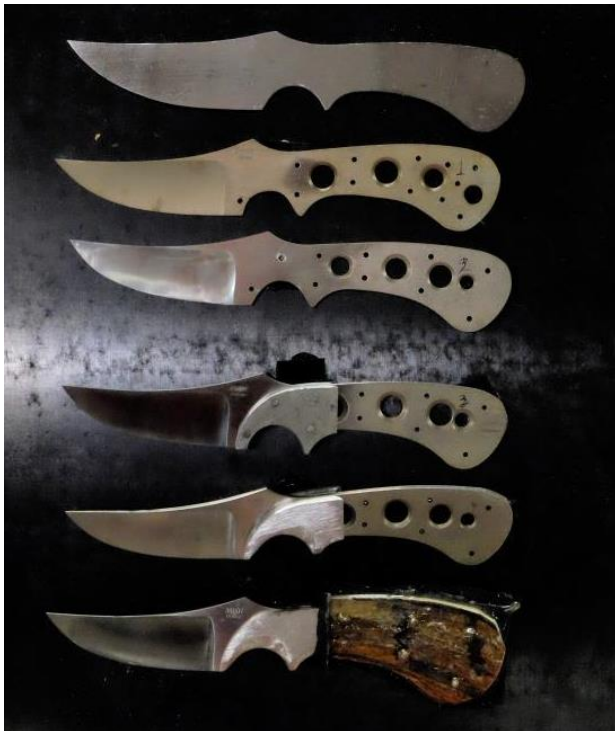
Here are the various stages of a Doug Ashby knife.
