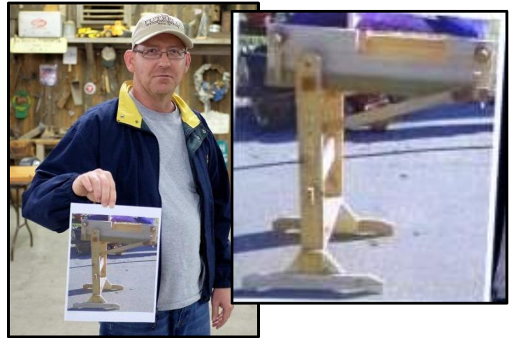
Gregory Futrell made this stand for the loom he showed off at the December meeting. He used mortise and tenon construction to make knockdown easy.
