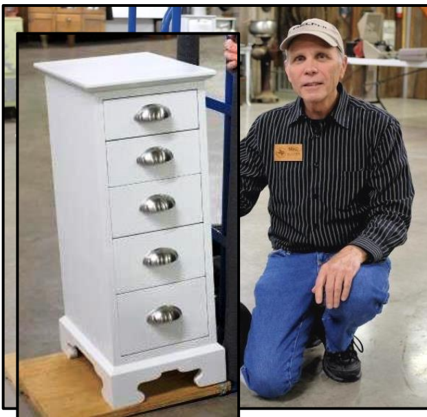
Mike Blazer made this small chest of drawers for his bathroom using hard and soft maple and Russian Baltic birch. He painted the chest due to the humidity in a bathroom.
