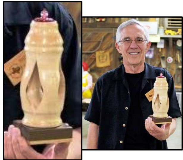
Richard Kenyon made this oil lamp out of maple and walnut using the inside/outside turning technique. He finished it using a Beal wax buffing process.
