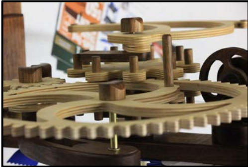
Smooth, equal sized teeth are a must
