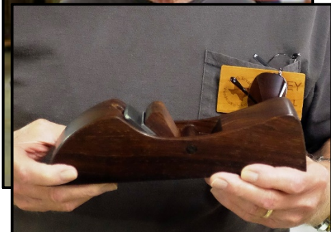
Sidney Futrell made this Enfield hand plane from Cocobolo for its weight. He added one pound of tungsten for even more weight.
