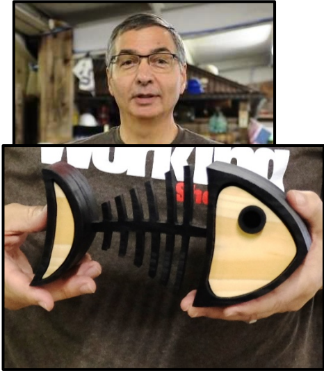
Ron Giordano made this fish-shaped band saw box out of a 1 x 6. He ebonized the black pieces using Behlen's dye topped with Minwax's ebony finish.
