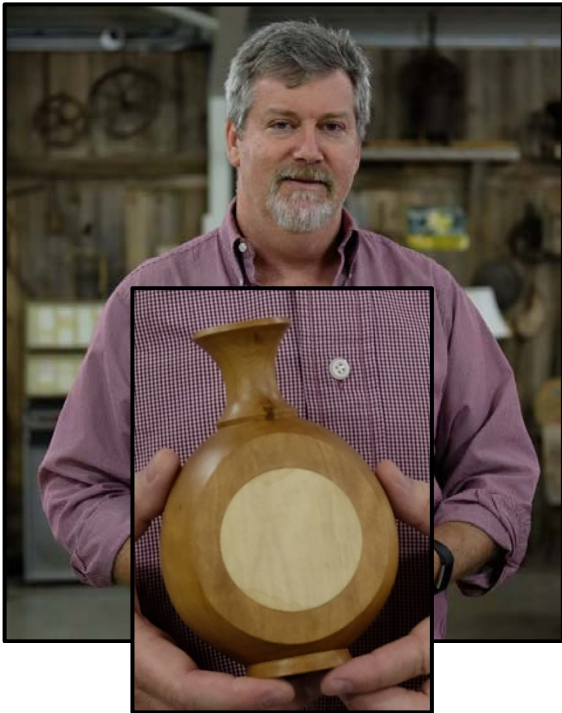
Steve Yauch turned this Jimmy Clewes designed water flask out of a single piece of cherry. The plug to seal the opening for hollowing the interior is made of tiger maple.
