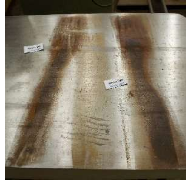
Tannin damage to cast iron jointer table.
