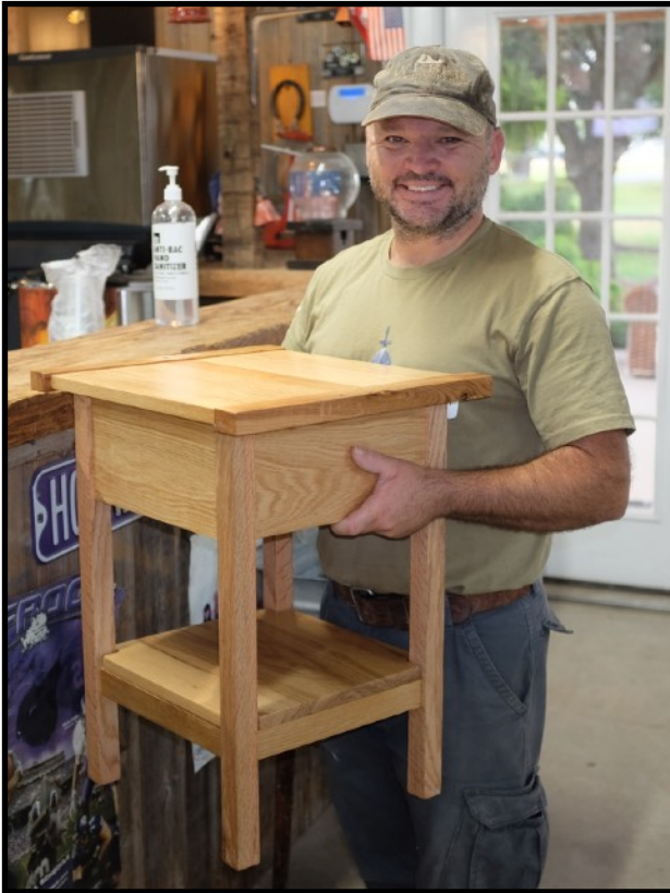
Phillip Weber built this side table in Stickley style out of scrap oak and cherry as a mock up for a later build with mahogany.
