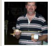
Steve Yauch made a vacuum chuck for the lathe using brass fittings and a gauge he brought from ebay.
