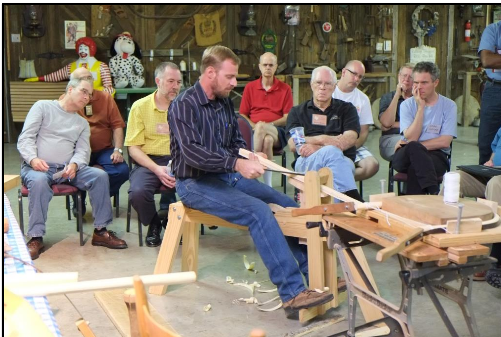
The shaping starts on the shaving horse
