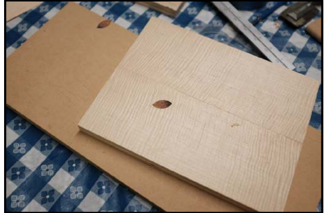
This shows a sand shaded leaf inserted into David's veneered sample.
