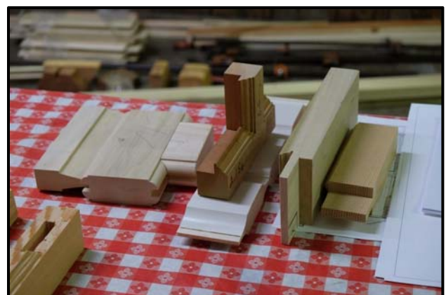
Figure 2: Examples of the profiles on the rails, stiles and panels.
