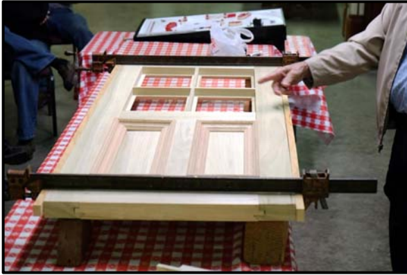
Figure 6: Assembled door with panels at bottom and muntins in place for glass lites.
