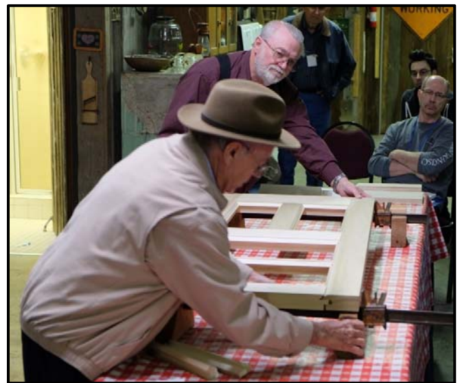
Figure 5: Use clamps on the rails to pull the door together and be sure to check for square!
