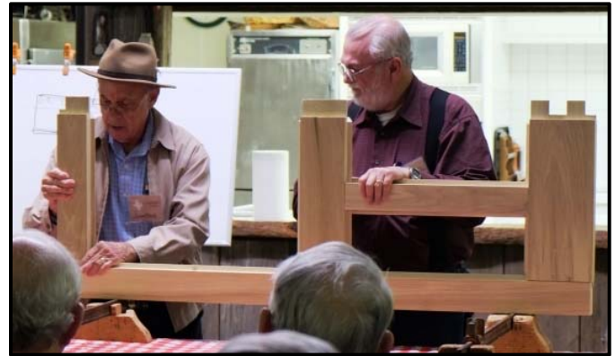
Figure 4: Lynn dry assembles his door with the help of a club member. Lynn says to always have help when assembling a door to be sure you have everything assembled before the glue sets.
