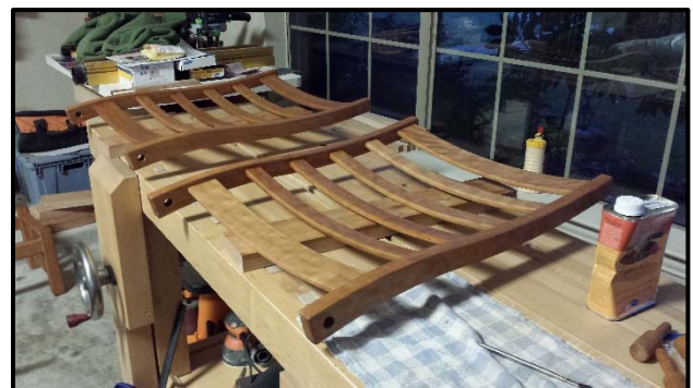
Bent laminations formed the chair back slats.
