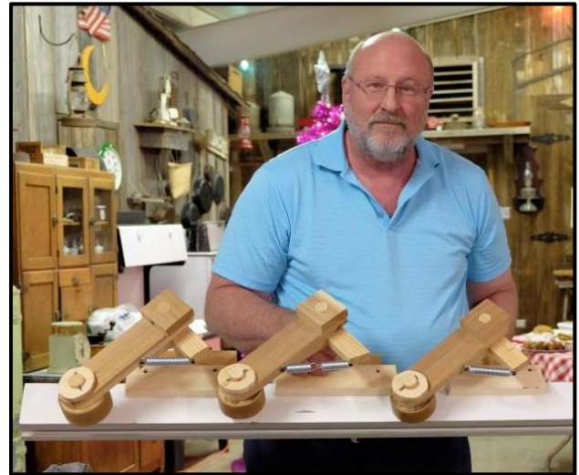
Scott Goldenberg showed off this router table fence/hold-down he made.
