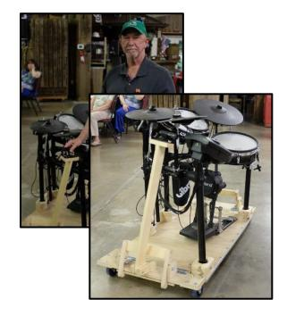
Fred Sawtelle likes to "jam" when he's not making sawdust, but taking his drum kit from gig-to-gig was a real pain so he put his woodworking skills to work and came up with this dolly system to safely transport the kit and easily move it into position.
