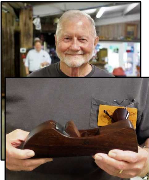
Sidney Futrell made this Enfield hand plane from Cocobolo for its weight. He added one pound of tungsten for even more weight.
