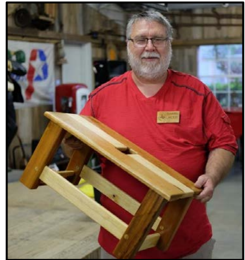
Dan Nilius made this exercise bench using pinned mortise and tenon joints. Scrap flooring was used for the top.
