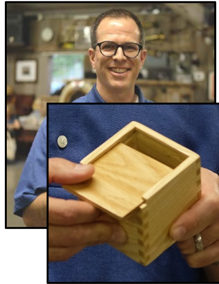
Britt Baumel made this box using finger joints and a sliding lid. He coated the ash with Armorseal.
