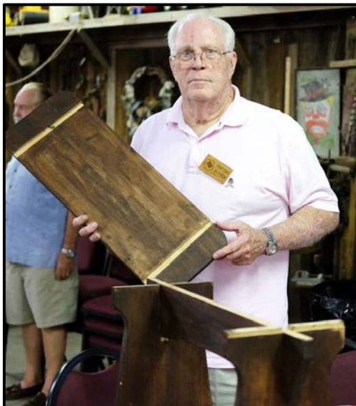
Wayne Bower made this table using sliding dovetails to secure the top.
