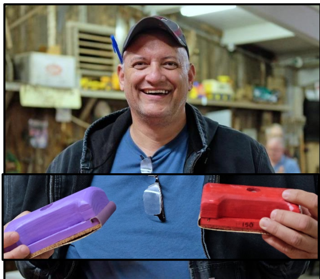
Carl Medina made these sanding blocks out of 2x4 scraps. Cork is glued to the bottoms and he painted them bright colors to make them visible in his shop.
