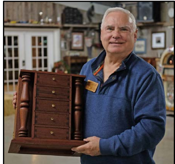
Gene Baugh made this jewelry box using mahogany. Joinery included finger joints on the drawers and mortise and tenons on the box. The finish is Danish oil.
