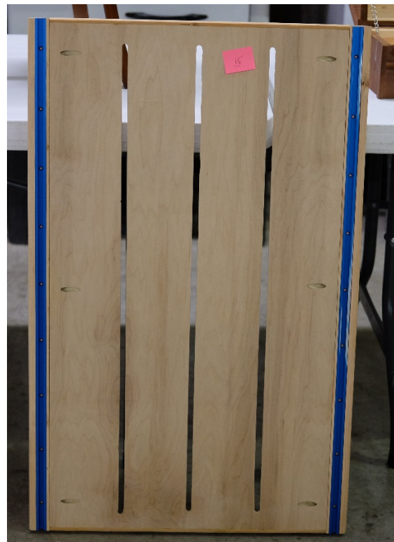
Swede Hanson made this clamp board for gluing up projects. The 2 x 4 frame has T-tracks for clamping along with the clamp slots in the center of the board.
