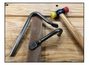
Michael uses holdfasts (fixture) by Gramercy Tools, which is used to hold a piece of work in place. The bench top (or other surface) has a 3/4" hole drilled in it. When the holdfast is hammered down, it wedges itself into the hole via spring action and holds a work piece firmly in place. To remove the holdfast, tap it on the bottom or back of the hold fast and it releases from the surface.
