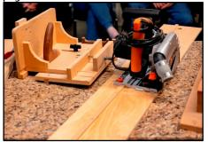
He also showed off his tenon jig and a kerf fitting jig used to cut "perfect" grooves, dados, and slots using a standard table saw blade – i.e. no need to use a dado blade. It is the perfect jig when making cross lap joints. The one Jerry showed is similar to the kerf maker in the following YouTube video: <u>https://www.youtube.com/watch?v=f</u> <u>NZWILPwOHI&t=340s</u>
