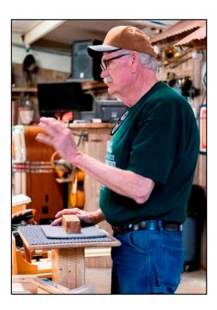
Nello Armstrong is more than a notch or two above average height which creates issues when he works at standard height benches, so he made this auxiliary table to raise his work to a comfortable height.
