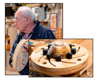
The "bumpers" adjust to the size of the bowl blank by loosening the wing nuts on the back and rotating the rings of plywood. The slots allow the bumpers to move at the same rate.
