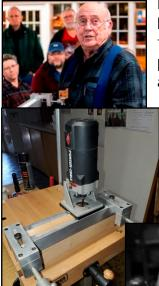
His first was a hinge mortising jig that is used with a palm router to accurately place door hinges.
