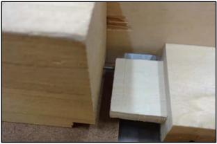
The advantages of this jig is that you use the blade height adjustment to get the exact thickness of the tenon to match your mortise. Another advantage is that with the stock laying down flat you don't have a long piece of stock sticking up in the air and trying to keep exactly perpendicular to the table. Steve Yauch's favorite jig is a cutoff sled that he uses for critical end cuts.
