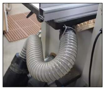
A clip fashioned from wire uses an existing bolt hole to help hold the hose in place.
