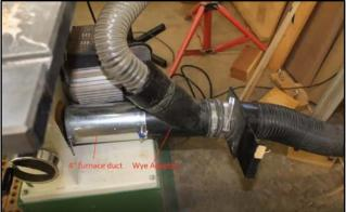
Note the 4" furnace duct to extend the port for the use of a wye instead of a Tee. He had the wye and didn't want to buy a Tee.
