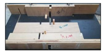
Joe Polich's favorite jig is a sled for cutting tenons. It makes it easy to cut the tenon to the exact size needed to fit the mortise and be perfectly centered. He cuts the mortise first using a Delta Mortising machine.
