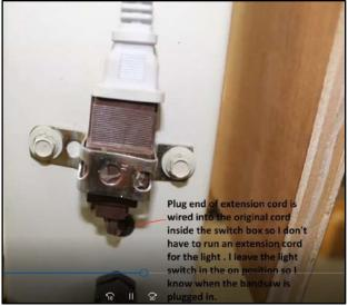
Another upgrade to his bandsaw was the led light that Gary Turman recommended. Rather than run an extension cord to power the light, Joe cut off the end of an extension cord and wired it into the original Rikon light cord. You can access the original cord by removing the switch plate on the front of the bandsaw. By not cutting off the plug, Joe can move the light to another location should the need arise.
