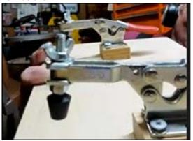
He also pointed out that many toggle clamps are now coming from overseas and can be too flexible, not allowing full clamp pressure. The Cadillac of toggle clamps is Destaco which are widely used in the tool and die trade.
