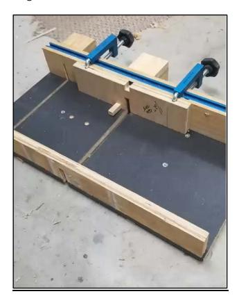
Jim has multiple plates for different size finger joints.
