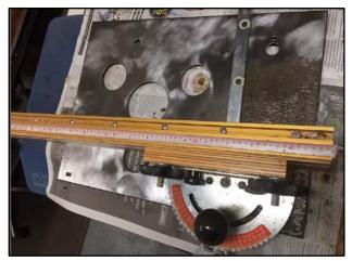
A second t-track on the top of the fence allows Steve to add hold-down fixtures.
