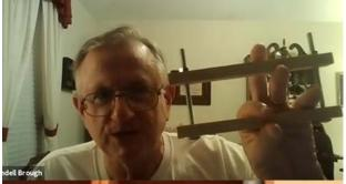
The jig is made from two pieces of 1/2" wood and two screws with nuts and washers. He places the stock for the ornament between the wood stretchers and tightens the screws to clamp it in place while he works on it.
