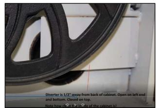
Notice the difference in the baffle in Joe's Rikon vs. Greg's and Jim's. Joe's is a solid piece that sets ½" off the back of the cabinet, is closed on the top and open on the left and bottom. The inside of his cabinet has always stayed dust free even before the new hose was added.
