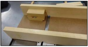
The stop block is adjustable to set the length of the tenon. A closer view of the stop block shows a small nail that the tenon stock is seated against.
