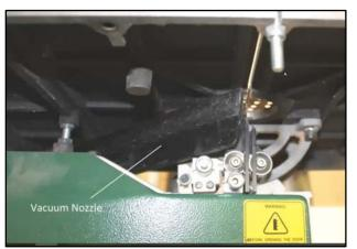
The nozzle keeps all dust from collecting around the blade guides and top of cabinet. Amazing difference!
