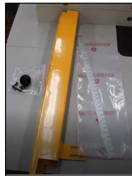
This is the upper bearing assembly with the two mounting blocks.
