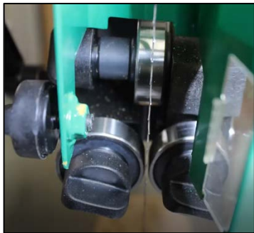
Upper bearing assembly adjusted for 1/2" blade.
