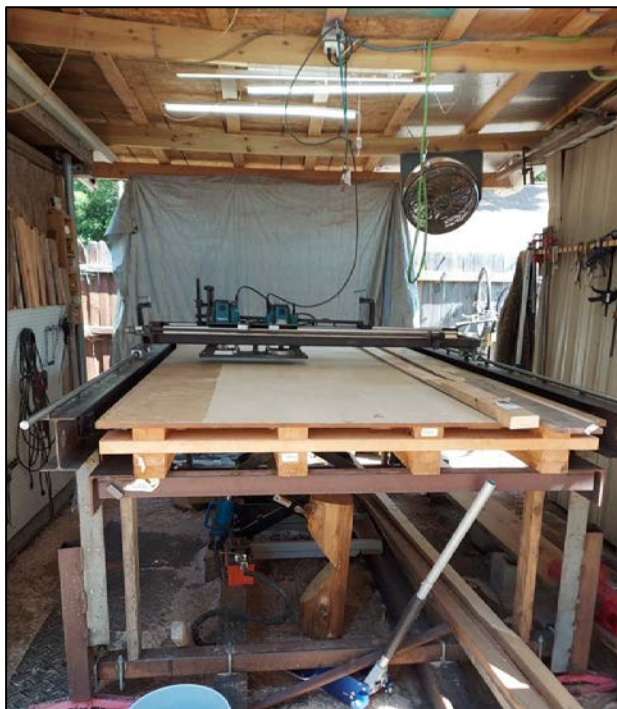
This is the machine Caleb built to flatten large slabs for tabletops
