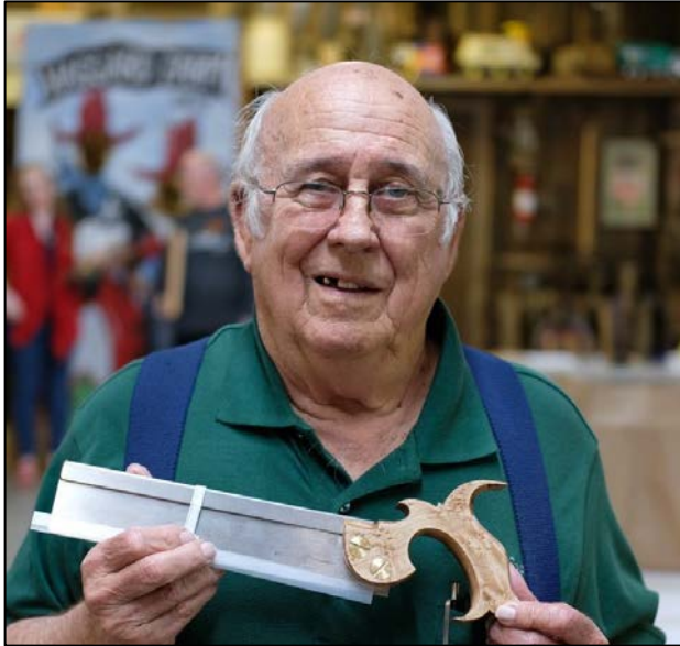
Gary Turman bought this old Disston dovetail saw at a yard sale. The teeth were broken and misshapen so Gary refiled all the teeth and replaced the straight handle with his own version of what a saw handle should be.
