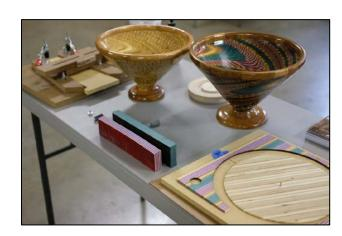
Small, thin slices are glued up to create blocks that would be cut into circles and glued up in layers. Jeff says this is a time-consuming operation and he made jigs to keep the blocks flat.
