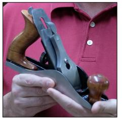
Brian O'Donnell brought in another hand plane that he has restored by repairing the broken handle and using electrolysis to remove the rust. It's a Stanley Defiance of the World War II era time.
