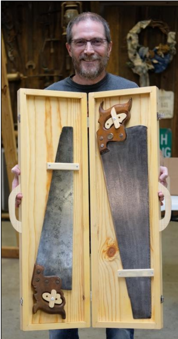
Michael Bosley put all his tools in a toolbox for travelling, but his saws wouldn't fit so he built this saw box over a weekend. It's finished with boiled linseed oil.
