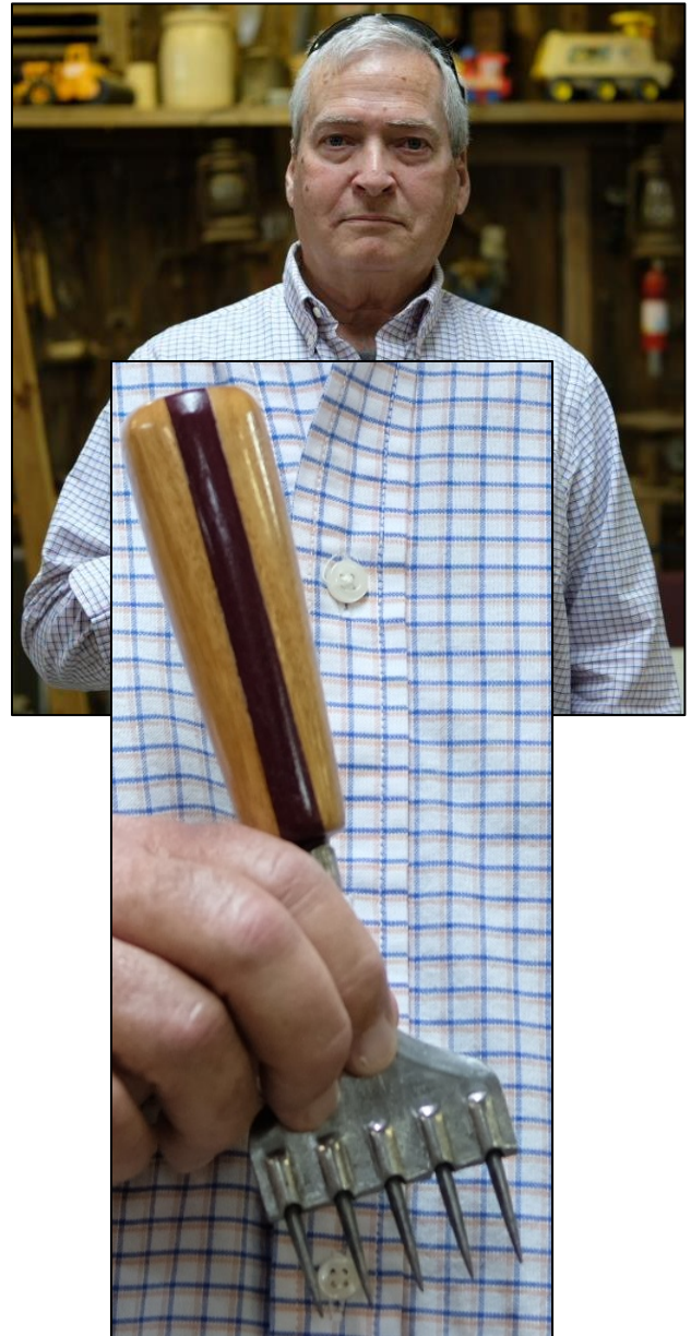
Kevin Pilgrim replaced the handle on his mother's old icepick. The original handle didn't fit her hand very well, so he made the replacement larger. He shaped it by hand because he doesn't have a lathe. His mother fell in love with the canary wood and the purple heart so that's what was used. The finish is an aerosol lacquer.
