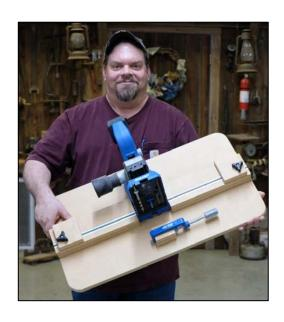
Roger McDaniel made this table to hold his Kreg pocket hole jig. It is fully adjustable and the Kreg jig can be removed if necessary.
