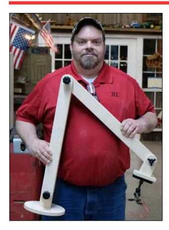
Roger McDaniel made this adjustable stand to keep his Bosch dust extractor in the right position. The stand easily moves around the bench and the arms can be adjusted to just about any needed position.
