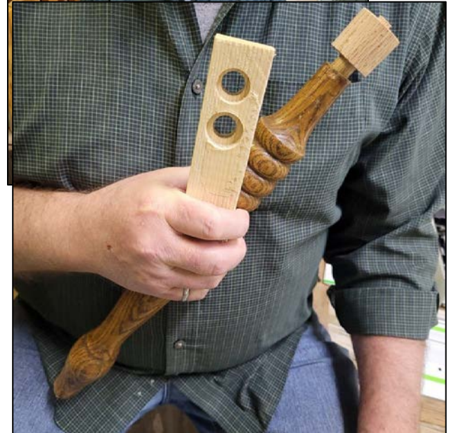
Steve Yauch repaired table legs for a Plano restaurant and came up with this jig to drill centered holes for dowels.
