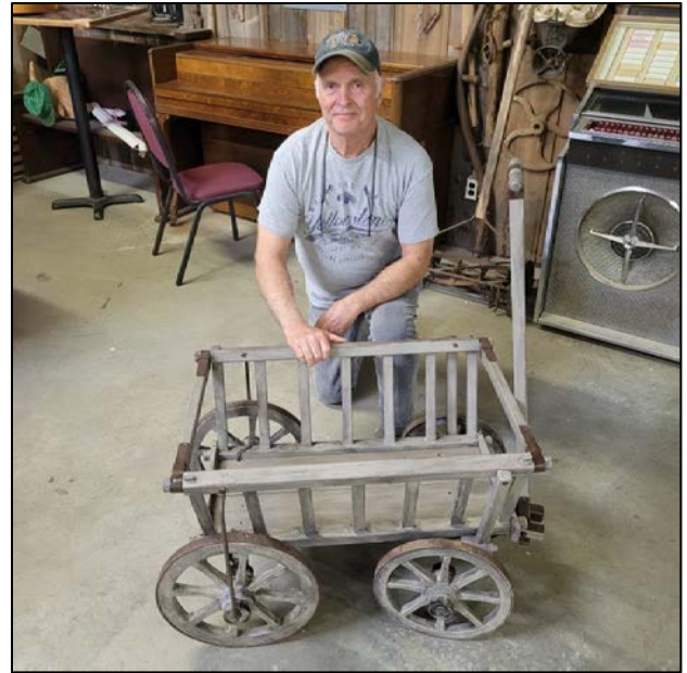
Bill Landis had to use all new wood to restore this antique wagon. Only the metal pieces are original. He used an antiquing technique to make the wood look old.
