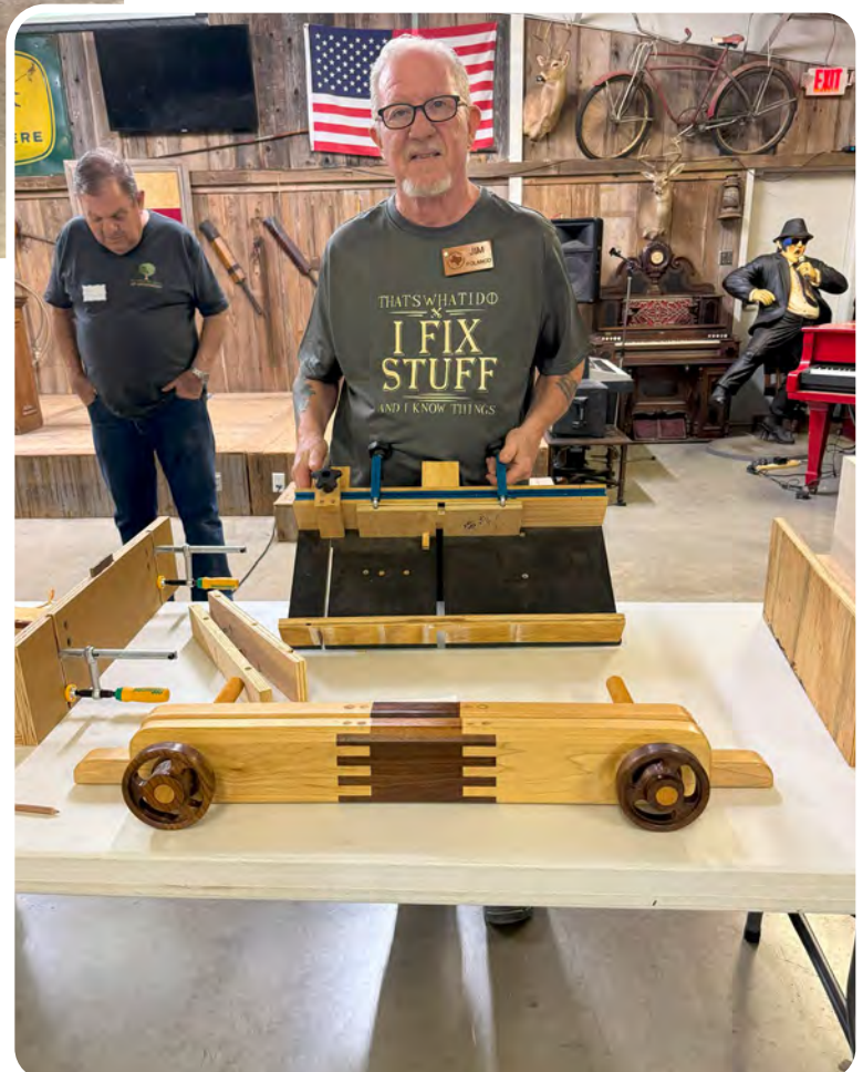
Jim Polanco crafted a Box Joint Jig and Moxon Vise out of Walnut and Maple.
