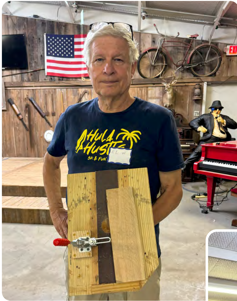
Ed Haluska created a Large Angled Hole Jig out of Scrap 2x12.
